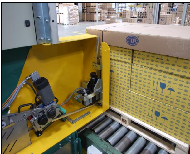
MH Head indexed onto side of pallet load for optimum strap tension to the load, head carriage stroke to load 500 mm
