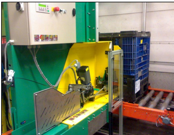
MH-VRB securing lids on re-usable bulk crates and is also suitable for most pallet strapping operations for loads with a minimum height of 350mm
