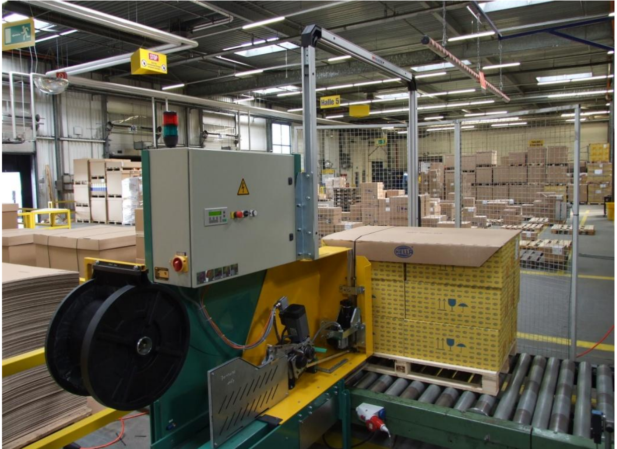
MH-VRB Side-Seal Machine shown in a high through-put production plant strapping palletised and packaged automotive components ready for shipment worldwide
