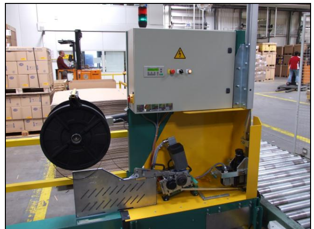
Set up of the Feeder and Sealer Modules with easy machine operator access and operations and for service work.
