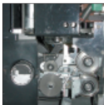
HB Strapping Head The cam-driven HB strapping head is designed for long operational life and requires virtually no maintenance.
