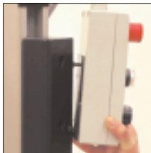
Easy control Setting Portable operator controls enable the strap cycle to be activated and adjusted from both sides of the machine.
